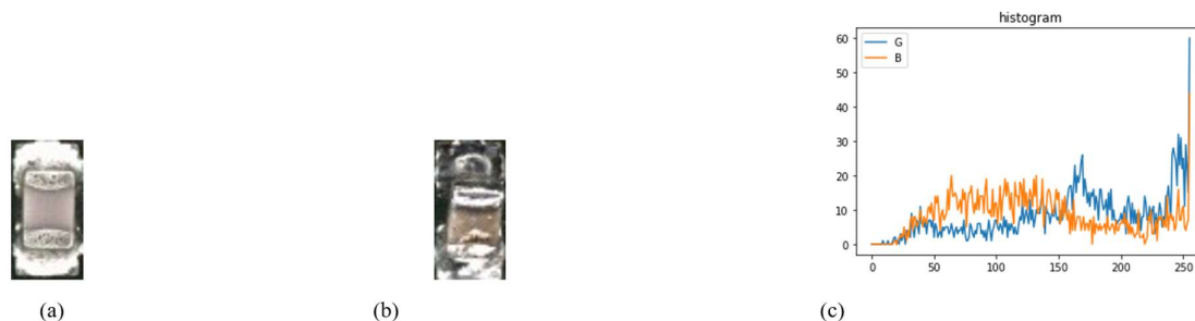
Figure 8. Histogram comparison for non-defective component with Tomb stoning defect component (a) Non-defective component (b) Tomb stoning component (c) comparison of grey level intensity of (a) & (b)
