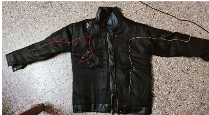
Fig 5. Inside wiring view of the of Safety Jacket
