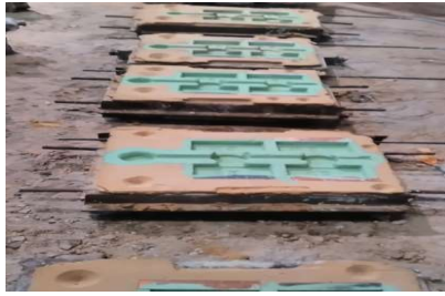
Figure. 2. (a) CO 2 process sand mold coated with zircon fluid ready for Pouring
