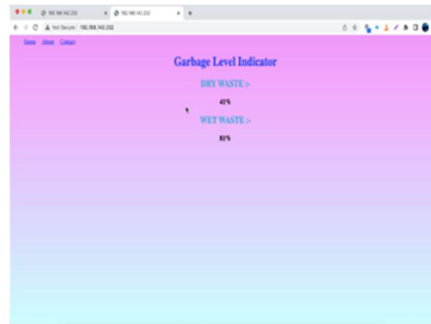
Fig.5.1: Real-time monitoring through local area network in a webpage (without internet)
