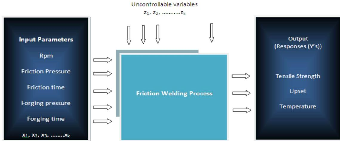
Figure 3.1 Block diagram of design of experiment
