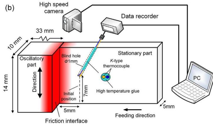
**Figure 2: Linear friction welding setup**
