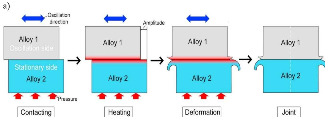
Figure 1: Friction Welding Trails
