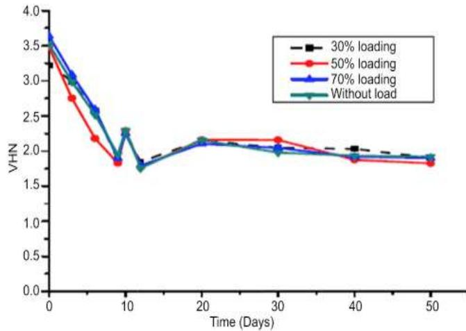
**Figure 3: Relationship of Vickers Hardness of Material with time**
