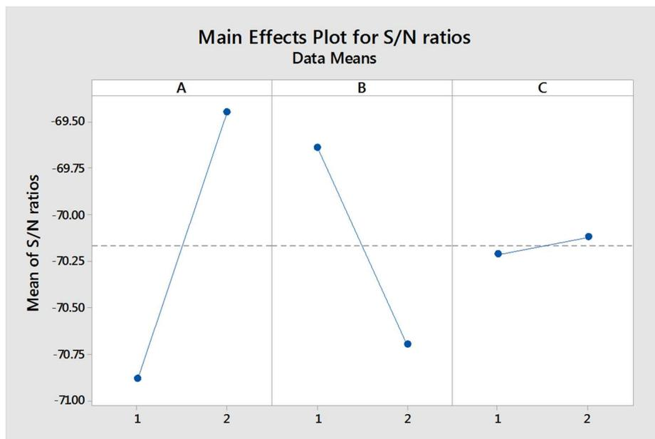
B. Fig.4.9 displays a major effects plot for the S/N ratio, demonstrating the optimum parameter combination for the traverse force.
