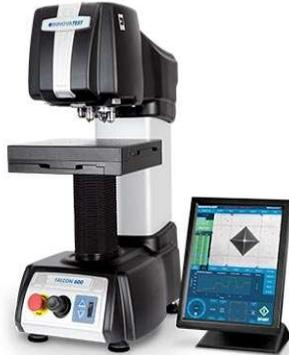
Vickers Micro Hardness Testing Machine
