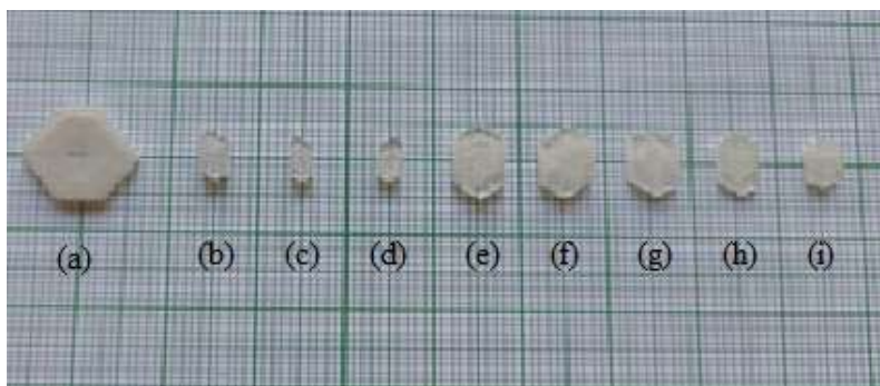
Fig. 3. Crystal habit of (a) TU; (b),(c) and (d) 0.5 M% OA doped TU; (e),(f),(g),(h) and (i) 1 M% OA doped TU
