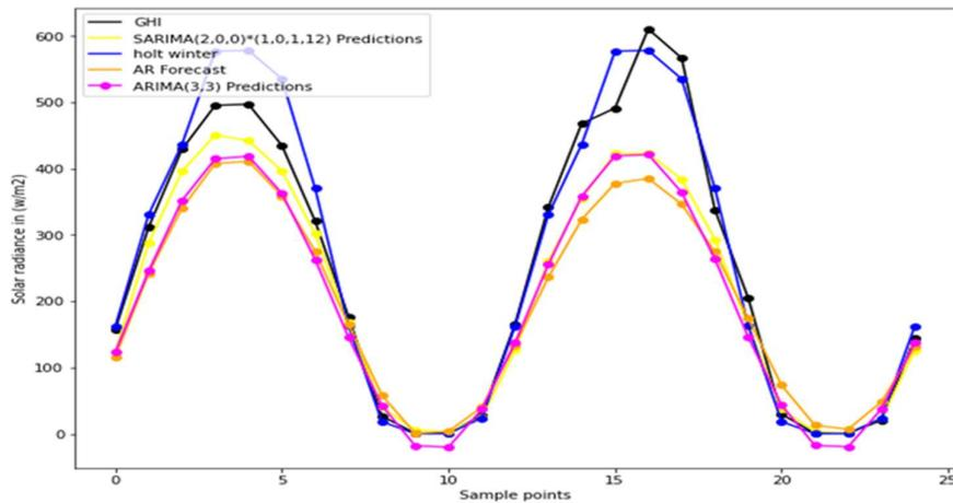
Fig 9 Solar radiation data on 30<sup>th</sup> December: 48 Hour ahead Forecasting
