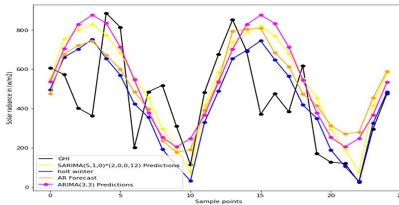
**Fig 7** Solar radiation data on 25<sup>th</sup> June 2021: 48 Hour ahead Forecasting
