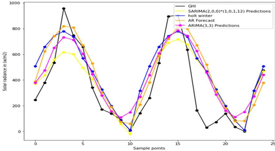
Fig 8 Solar radiation data on 30<sup>th</sup> August 2021: 48 Hour ahead Forecasting
