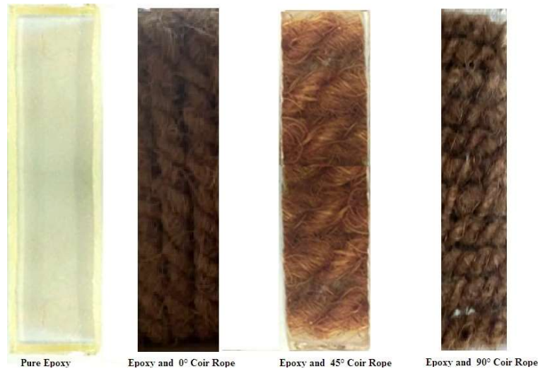
Figure 2: Sample preparation at different orientation of coir rope in epoxy
