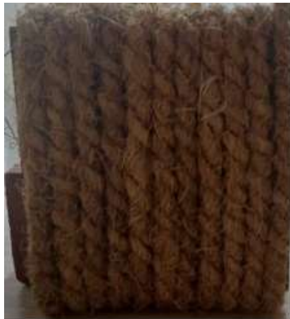
Figure 1: Wrapping coir rope around the mould
