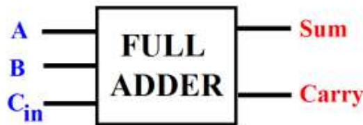
Figure 2: Block diagram of 1-bit Full Adder
