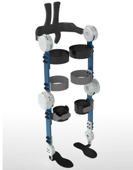
Figure 2: CAD model of lower limb exoskeleton robot.
