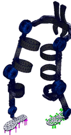
Figure 3: partition into grids and loading of the exoskeleton of the lower leg
