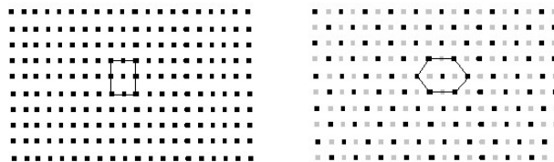
Figure 7: Rectangular grid and hexagonal grid reproduced using alternate pixel suppression method
